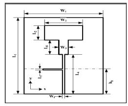
Figure 1: Design of a T-Shaped Antenna
