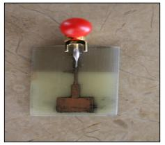
Figure 6: PCB Design of a T shaped Antenna
