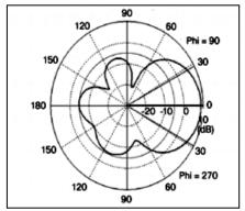
Figure 5: Elevation plane pattern on FR4
