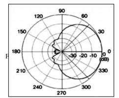
Figure 5: Elevation plane pattern on FR4
