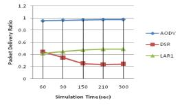
Fig.8 Packet delivery Ratio vs. Simulation Time
