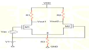
Fig. 1 Differential Amplifier with source degeneration
