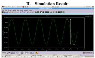
Fig.5 Hspicesimulation of Simple Differential OTA
