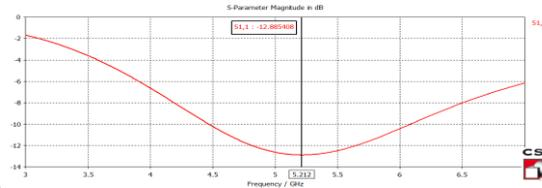
Figure 2. S-parameter representation [ $h=18$ ,  $hp=10$ ,  $S=50$ ,  $L_d=11$ ,  $\epsilon_r=4$ ,  $r=0.635$ ,  $R=2.124$ ] All dimensions are in mm
