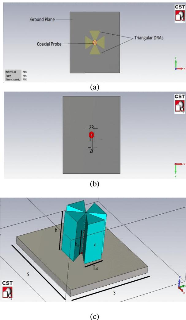
Figure 1. Geometry of the Four Triangular DRA with Ground Plane (a) Top View (b) Bottom view (c) Side View [ $h=18$ ,  $h_p=10$ ,  $S=50$ ,  $L_d=11$ ,  $\epsilon_r=4$ ,  $r=0.635$ ,  $R=2.124$ ] All dimensions are in mm
