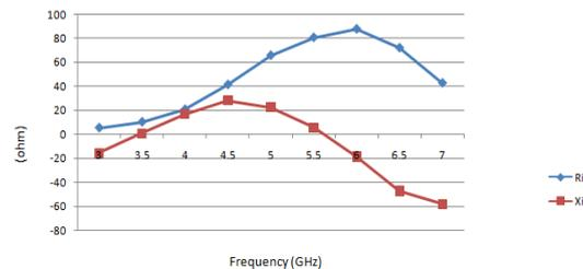
Figure 7. Simulated input impedance [h=18, hp=10, S=50, L<sub>d</sub>=11, ε<sub>r</sub>=4, r=0.635, R=2.124] All dimensions are in mm
