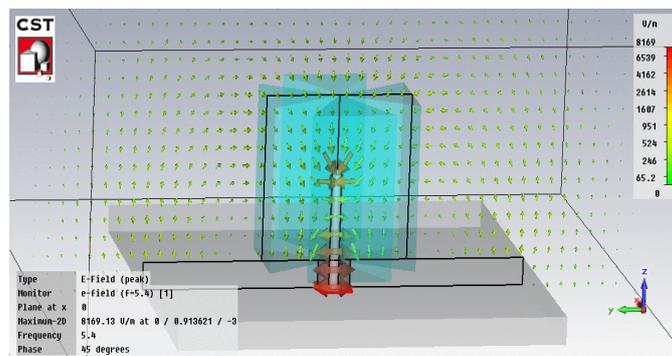
Figure 5. E-Field distribution at 5.4 GHz [h=18, hp=10, S=50, L<sub>d</sub>=11, ε<sub>r</sub>=4, r=0.635, R=2.124] All dimensions are in mm
