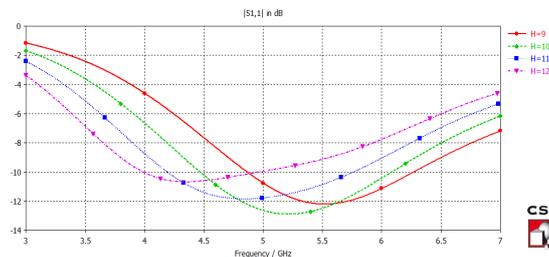
Figure 10. Variation of S-Parameter with variation in hip [h=18, S=50,  $L_d=11$ ,  $\epsilon_r=4$ , r=0.635, R=2.124] All dimensions are in mm.
