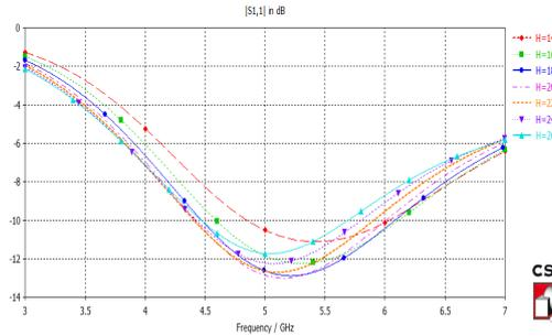
Figure 9. Variation of S-Parameter with variation in h with [hp=10, S=50,  $L_d=11$ ,  $\epsilon_r=4$ , r=0.635, R=2.124] All dimensions are in mm
