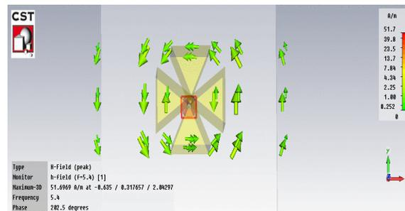
Figure 6. H-Field distribution at 5.4 GHz [h=18, hp=10, S=50, L<sub>d</sub>=11, ε<sub>r</sub>=4, r=0.635, R=2.124] All dimensions are in mm
