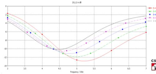
Figure 8. Variation of S-Parameter with variation in  $\epsilon_r$  [h=18, hp=10, S=50,  $L_d=11$ , r=0.635, R=2.124] All dimensions are in mm
