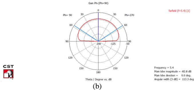
Figure 4. (a)E-Plane (Electric Monopole), (b) H-Plane (Horizontal Magnetic Dipole) [h=18, hp=10, S=50, L<sub>d</sub>=11, ε<sub>r</sub>=4, r=0.635, R=2.124] All dimensions are in mm
