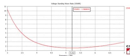
Figure 11.VSWR for Four Triangular DRAs [h=18, hp=10, S=50, L<sub>d</sub>=11, ε<sub>r</sub>=4, r=0.635, R=2.124] All dimensions are in mm
