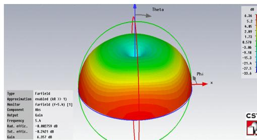
Figure 3.3-D view simulated gain of the triangular dielectric resonator [ $h=18$ ,  $hp=10$ ,  $S=50$ ,  $L_d=11$ ,  $\epsilon_r=4$ ,  $r=0.635$ ,  $R=2.124$ ] All dimensions are in mm
