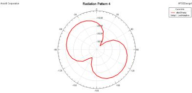
Figure 13: Radiation pattern of antenna (xz-plane)
