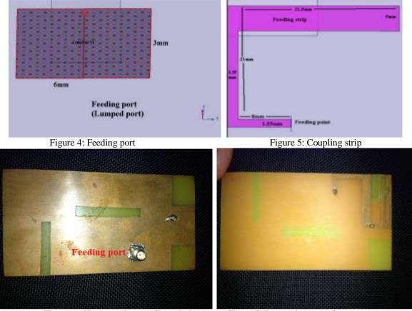
Figure 6: Hardware image (Ground plane)
