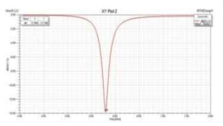
Figure-5.1.1: Return Loss (in db) without Dual FSS FSS
