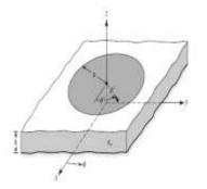
Figure 2.1: Geometry of Circular Patch Antenna.
