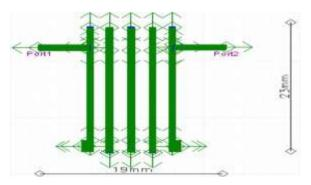
Figure 1. The EM model of bandpass filter
