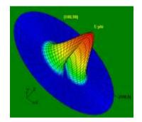
Figure 8: H-Plane (3D View) Radiation Pattern for slotted antenna at 9.54GHz
