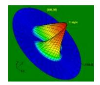
Figure 7: E-Plane (3D View) Radiation Pattern for slotted antenna at 9.54 GHz
