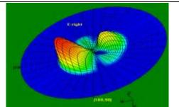
Figure 11: E-Plane (3D View) Radiation Pattern for slotted antenna at 12.90 GHz
