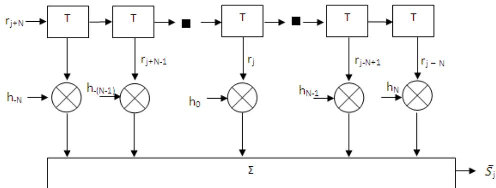
**Figure 15: Transversal Filter equalizer (Schwartz, P49)**
