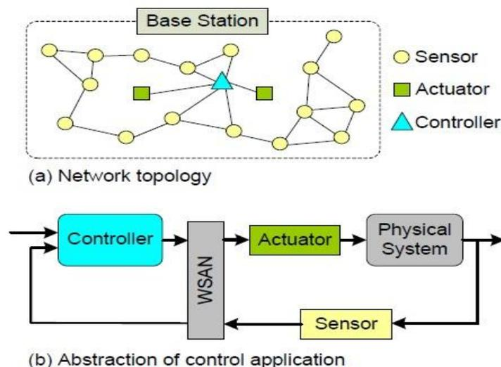
**Fig.2. WSN Architecture with explicit controllers.**
