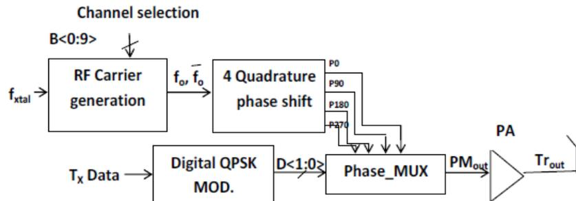
Fig.9 QPSK RF Transmitter
