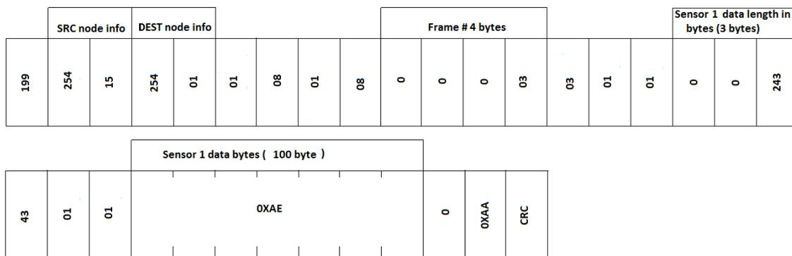
**Fig. 5** Proposed Bit frame format for One single zone of Telecom applications
