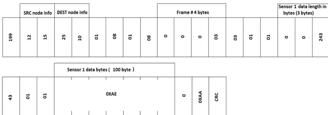
**Fig. 7 Proposed Bit frame format for Two different zones of Telecom applications**
