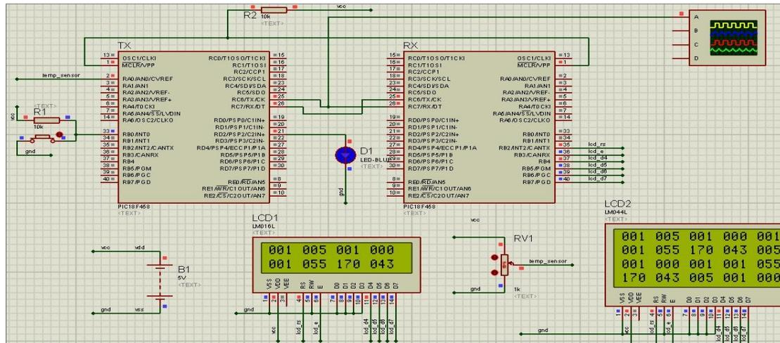
Fig. 8 shows the result snap shot taken from Proteus circuit simulation program with actual frame for the proposed bit frame generation for Telecom application
