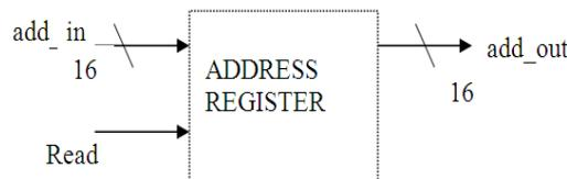
This is a 32-bit address register used for addressing the memory location. The memory is fetched from the location pointed by the address register. The address register combines with the page address and is passed to the memory. This unit takes a 32-bit address as input 'add\_in' and based on the selection addresses the particular memory location.
