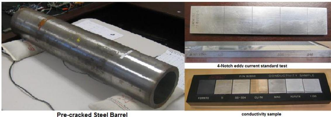
FIGURE 2. Pre-slot steel barrel (Left) and the 4-Notch EC standard test block and conductivity sample (Right)
