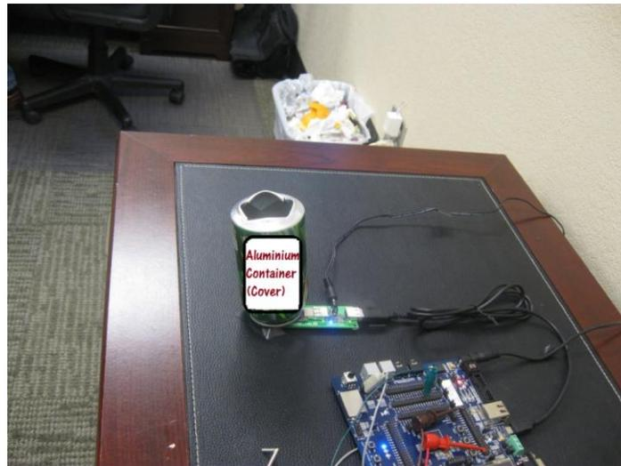
**FIGURE 6.** Picture of aluminum can which is covering instrument transceiver antenna
