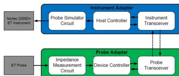
**FIGURE 1.** Wireless ET System Block Diagram
