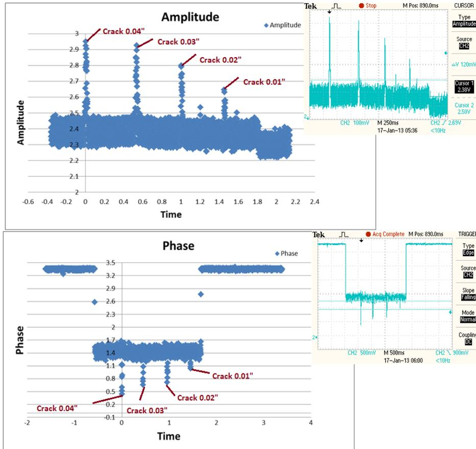
FIGURE 4. Amplitude (Top) and phase (Bottom) change signals detected with the impedance measurement circuit using 4-Notch eddy current standard test block
