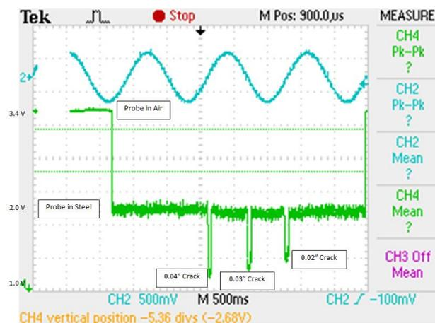
FIGURE 3. Probe Simulator Circuit I/O Signal Diagram
