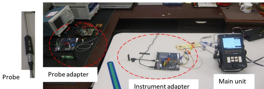
FIGURE 5. Basic wireless experimental system setup
