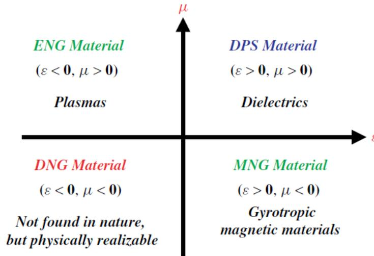
Fig. 1. Metamaterial classification based on  $\epsilon - \mu$  [1]
