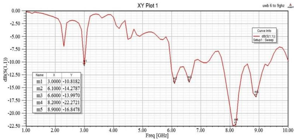
**Fig.9.** S11 verses frequency response after modification in ground structure.
