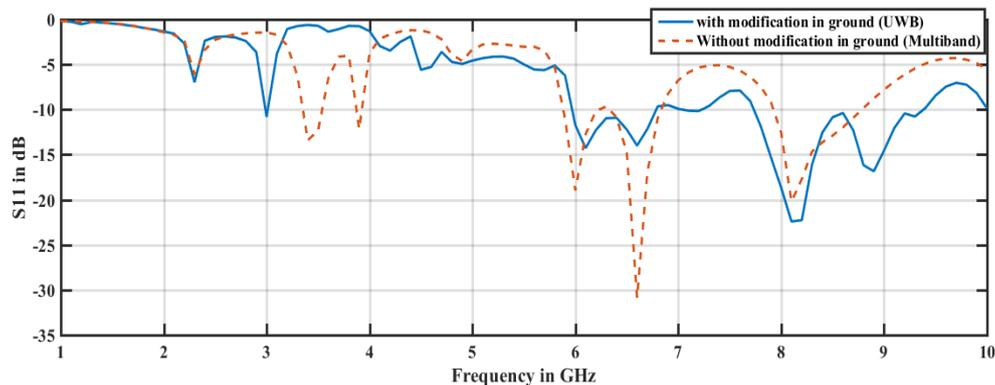
**Fig. 10** comparative results before and after modification of ground structure with SRR
