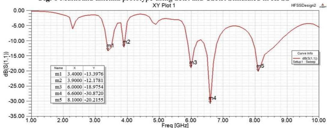
Fig.7. S11 versus frequency response for antenna
