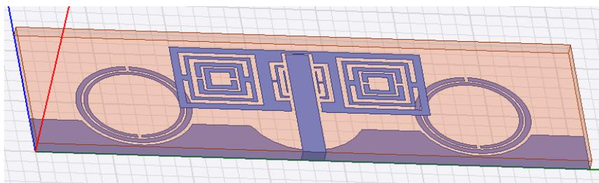
Fig. 6 Multiband antenna prototype using SRR and CSRR Simulated in HFSS
