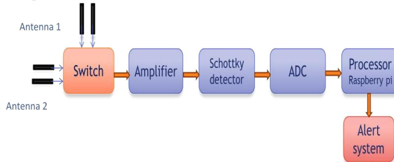
Fig:1. System Block Diagram
