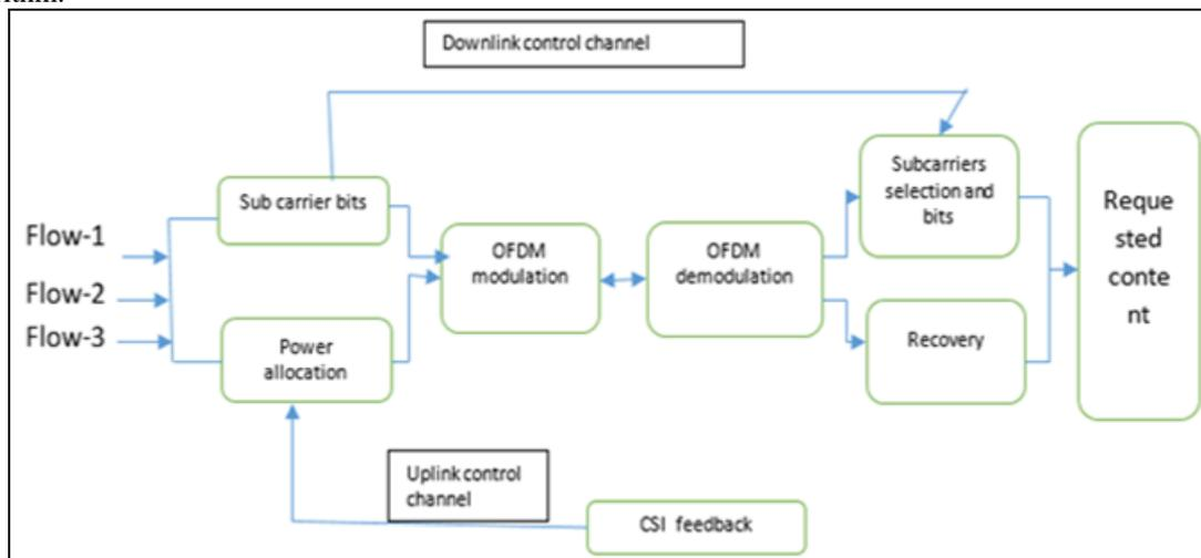
Fig.3: Block Diagram of multicast system model in OFDMA system.
