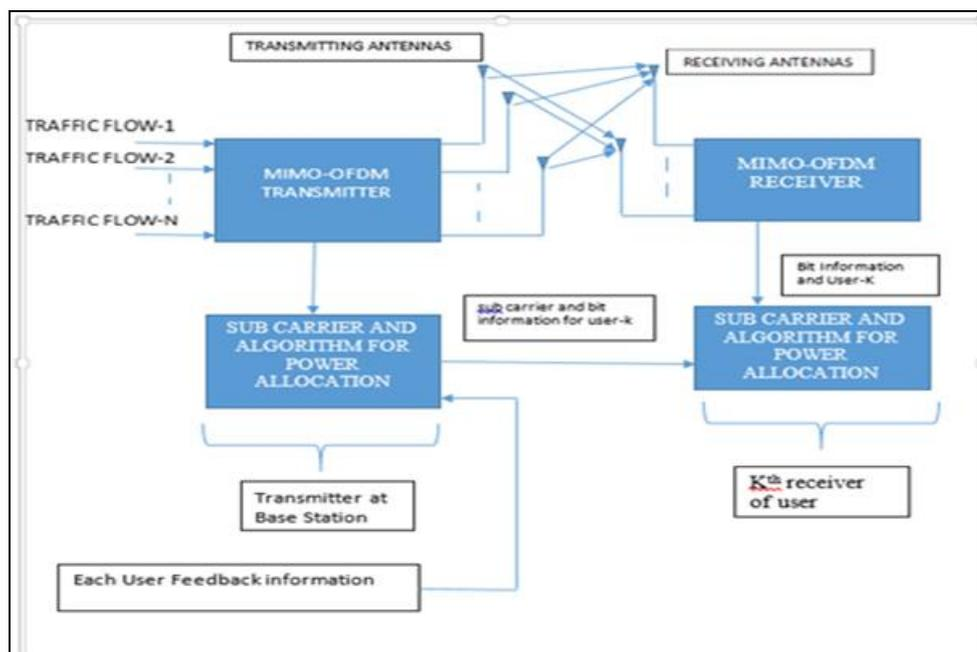
**Fig.2:** Block diagram of MIMO-OFDM system
