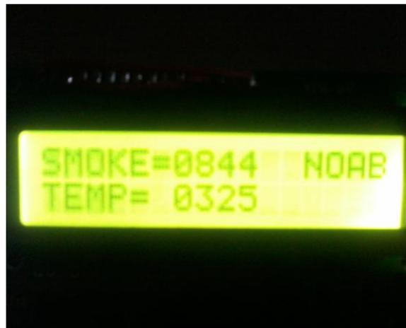
**Fig.9** The System Detected Smoke And Temperature Readings Displayed On The Lcd Display
