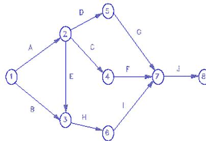
Fig.1: CPM Network Diagram
