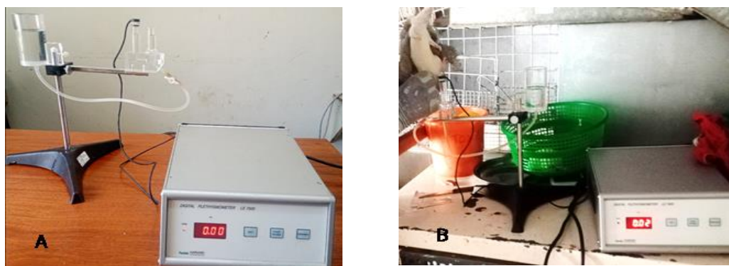
Figure 1.1: photogram showing: A calibrations of plethysmometer, B ; showing how to measure of hind limbs volumes of the wistar rat
