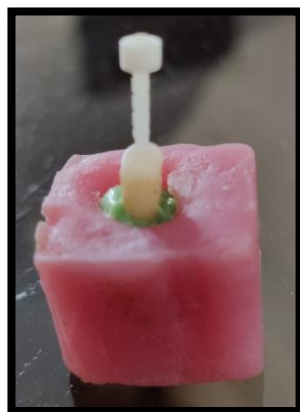
FIGURE 3: SAMPLES WERE MOUNTED ON SELF-CURING ACRYLIC BLOCKS
