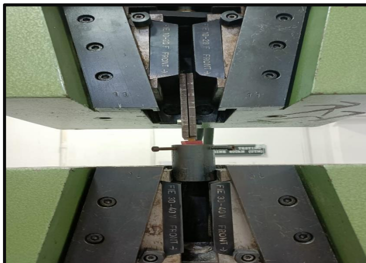
FIGURE 4: PULL OUT BOND STRENGTH EVALUATION DONE WITH UNIVERSAL TESTING MACHINE
