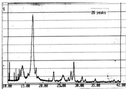
Fig. VII: X-RAY DIFFRACTION PATTERN OF STRUVITE
