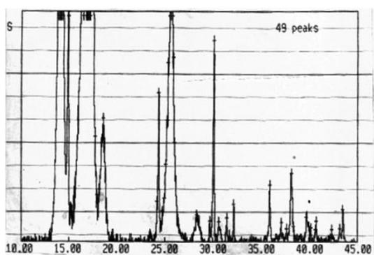
Fig. III : X-RAY DIFFRACTION PATTERN OF STRUVITE + HYDROXYAPATITE+ WHEWELLITE
