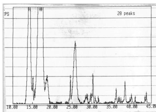
Fig. VI: X-RAY DIFFRACTION PATTERN OF WHEWELLITE+ WEDDELLITE
