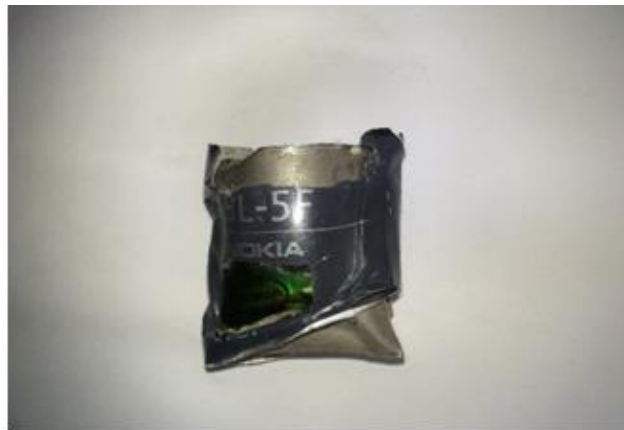
Figure 1. Nokia cell phone battery after explosion.
