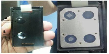
Figure 1 : TLD Chipsconsisting Li-F formeasurement of A) Deep dose B) Shallow dose
