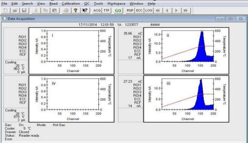
Figure 2: TLD Glow curve obatined using TLD 4500 reader
