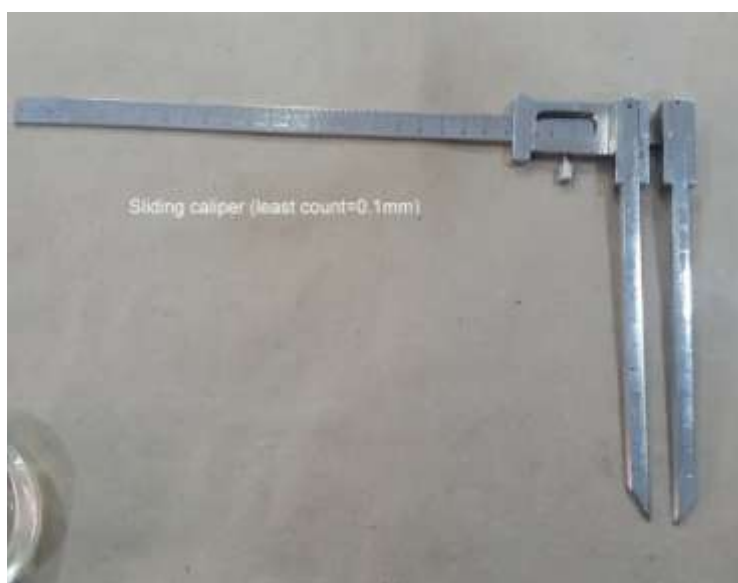
Fig-2: Slide callipers used for measuring distance of mandibular foramen from various landmarks
