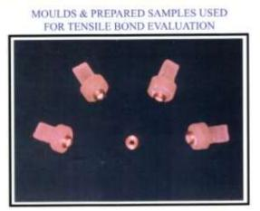
Fig-1. samples embedded in resin blocks.
