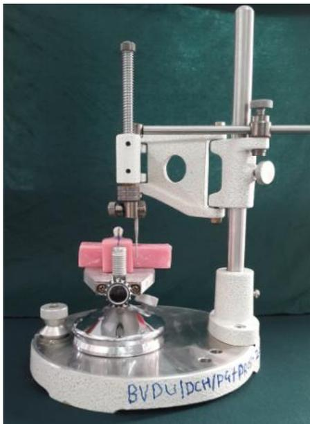
**Fig 2:** Surveyor used to achieve parallelism.
