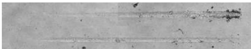
Figure 4 Scratches in composite material (CLSM image)
