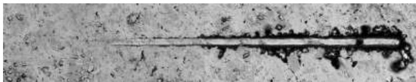
Figure 3 Scratches in dental amalgam (CLSM image)
