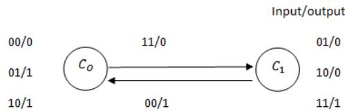
Fig. 3 Sequential Adder
