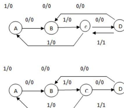
Fig. 4 Sequential Detector
