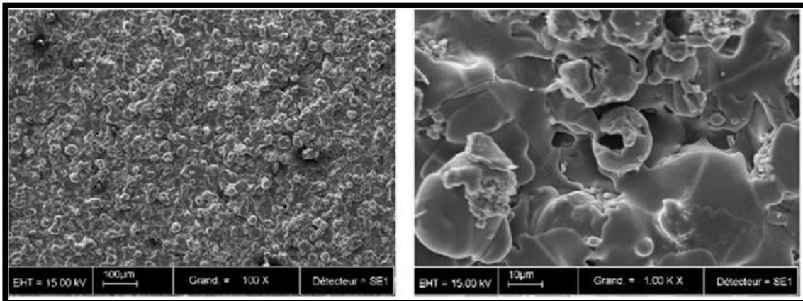
Scanning electron micrographs of a plasma-sprayed hydroxyapatite coating surface
