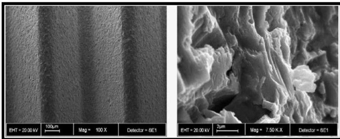
Scanning electron micrographs of a TiO<sub>2</sub> blasted surface
