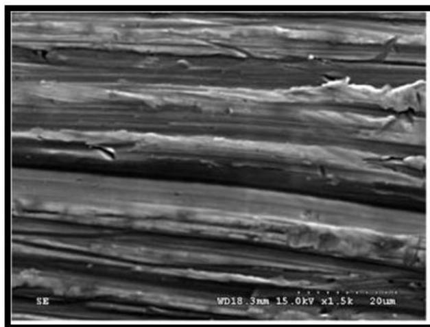
Scanning Electron Micrograph of Turned or Machined Dental Implant Surface
