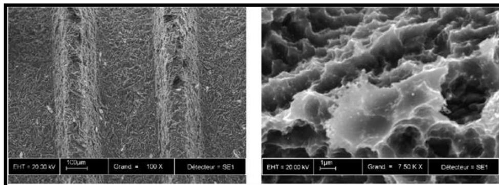
Scanning electron micrographs of an SLA surface on Titanium dental implant
