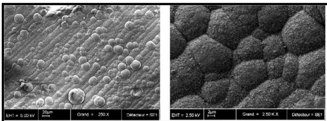
Scanning electron micrographs of a biomimetic calcium phosphate coating
