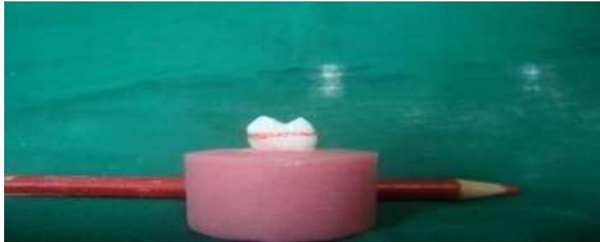
Fig. 1. Teeth mounted in autopolymerizing resin.
