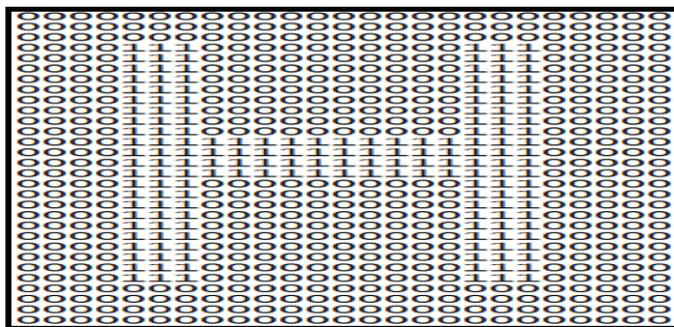
Fig-5. The letter 'H' after thresholding and binarisation
