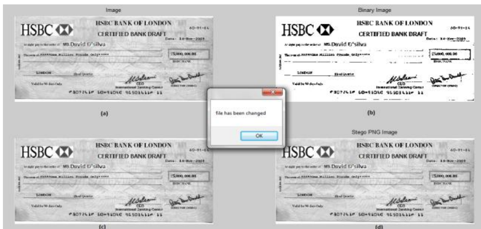
Fig. 6 Authentication result of a document image of a Cheque in the form of PNG tampered with image editor. (a) Original cover image-(edited one). (b) Binary-like of edited image. (c) Alpha plane of edited image. (d) Edited image in Stego PNG format.
