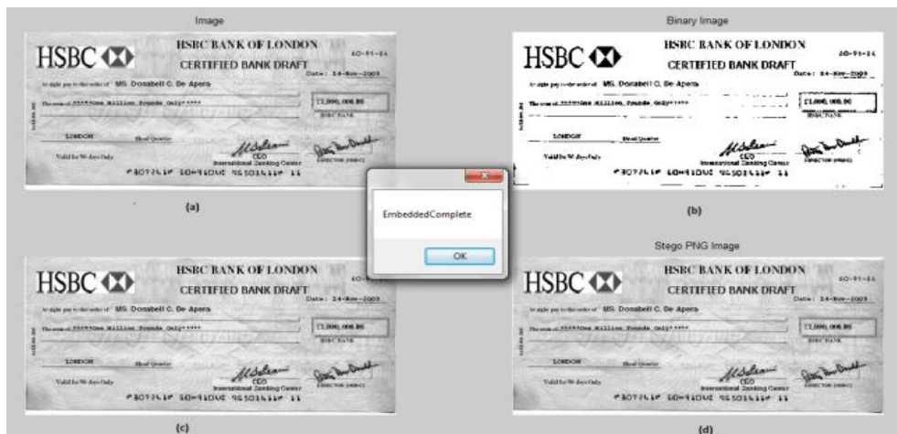
Fig. 5 Authentication result of an image of a Cheque in PNG format (a) Original cover image. (b) Binary-like of original image. (c) Alpha plane of original image. (d) Original image in Stego PNG format.
