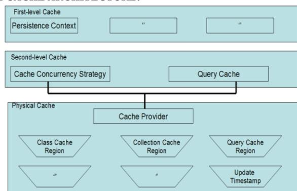
Figure 2 : Two-level cache architecture
