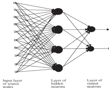
**Fig.** fully connected feed forward with one hidden layer and one output layer.
