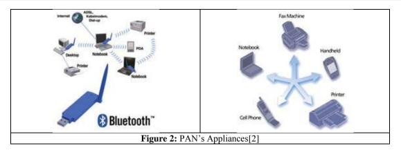
*Bluetooth:* Bluetooth is an engineering specification for wireless personal area networks (PANs), also known as IEEE 802.15.1. Bluetooth afford a way to connect and exchange information between devices such as personal digital assistants (PDAs), cell phones, PCs, laptops, digital cameras, printers, and video game consoles via a secure, globally unlicensed short-range radio frequency.
