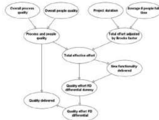
Figure 2 : A simplified version of the MODIST model USING THE BAYESIAN NET FOR DECISION SUPPORT
