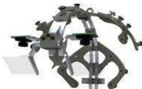
Figure 9: EEG signal acquisition system combined with eye tracking.
