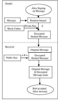
FIGURE.1 New Digital Signature Architecture
