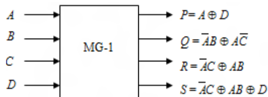
Figure 5: Block diagram of a 4x4 MG-1 Gates
