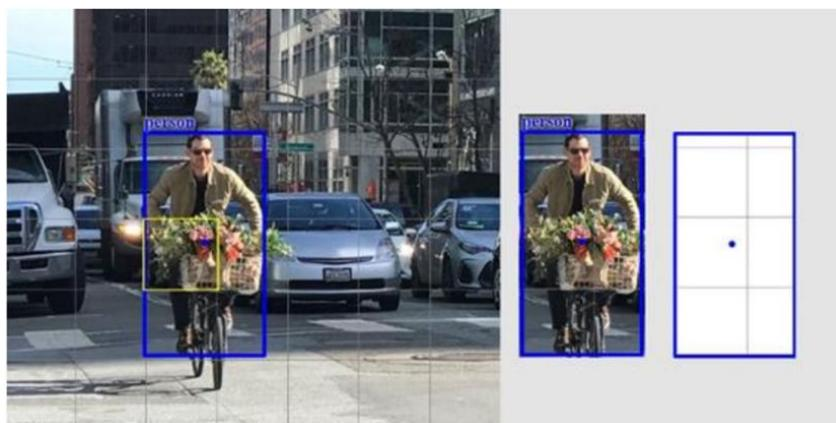
Figure 10. YOLO divides images into grid cells.
