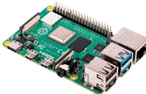
**Figure 1.** Raspberry Pi 4 Model B.
