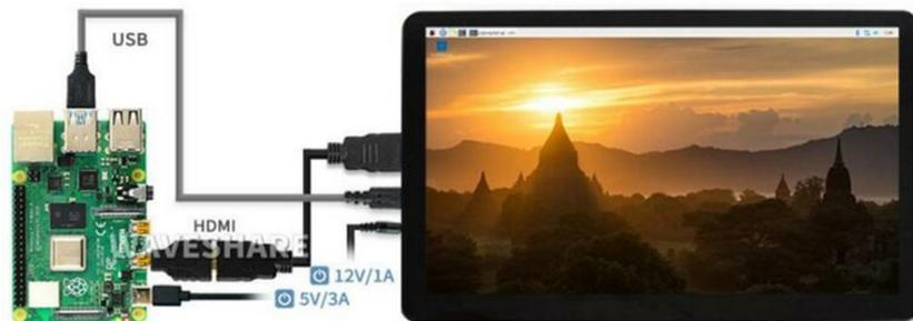
**Figure 5.** Connecting touch screen to Raspberry Pi 4B.
