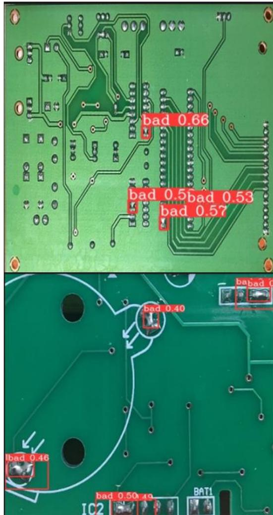
Figure 14. Detecting short solder joints.
