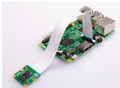
**Figure 6.** Connecting camera module to Raspberry Pi 4B.
