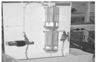
Figure 9. The cascaded tanks.
