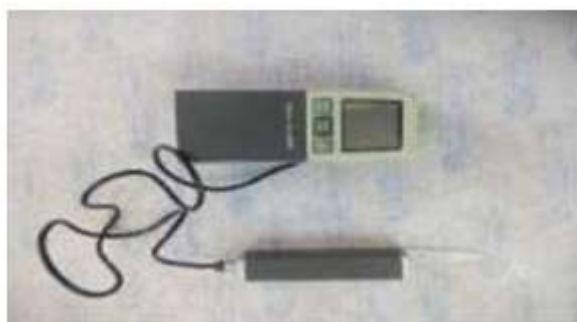
Figure 4. Mitutoyo surface roughness test instrument
