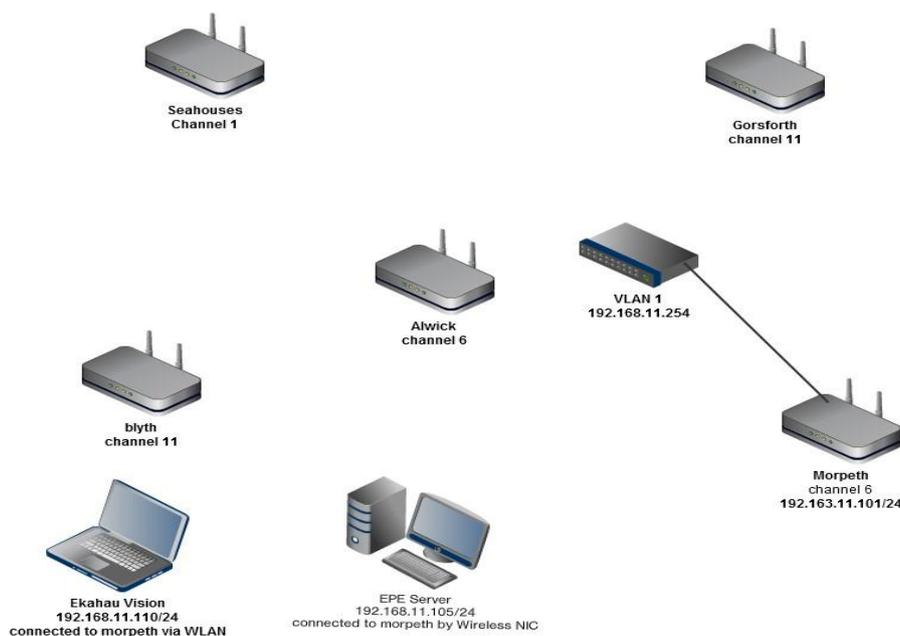
Fig 1. WLAN Network infrastructure for experiments
