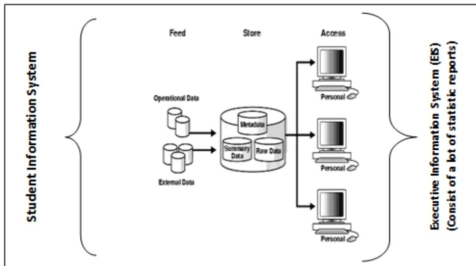
*Figure -2- Architecture of data repository of EIS*
