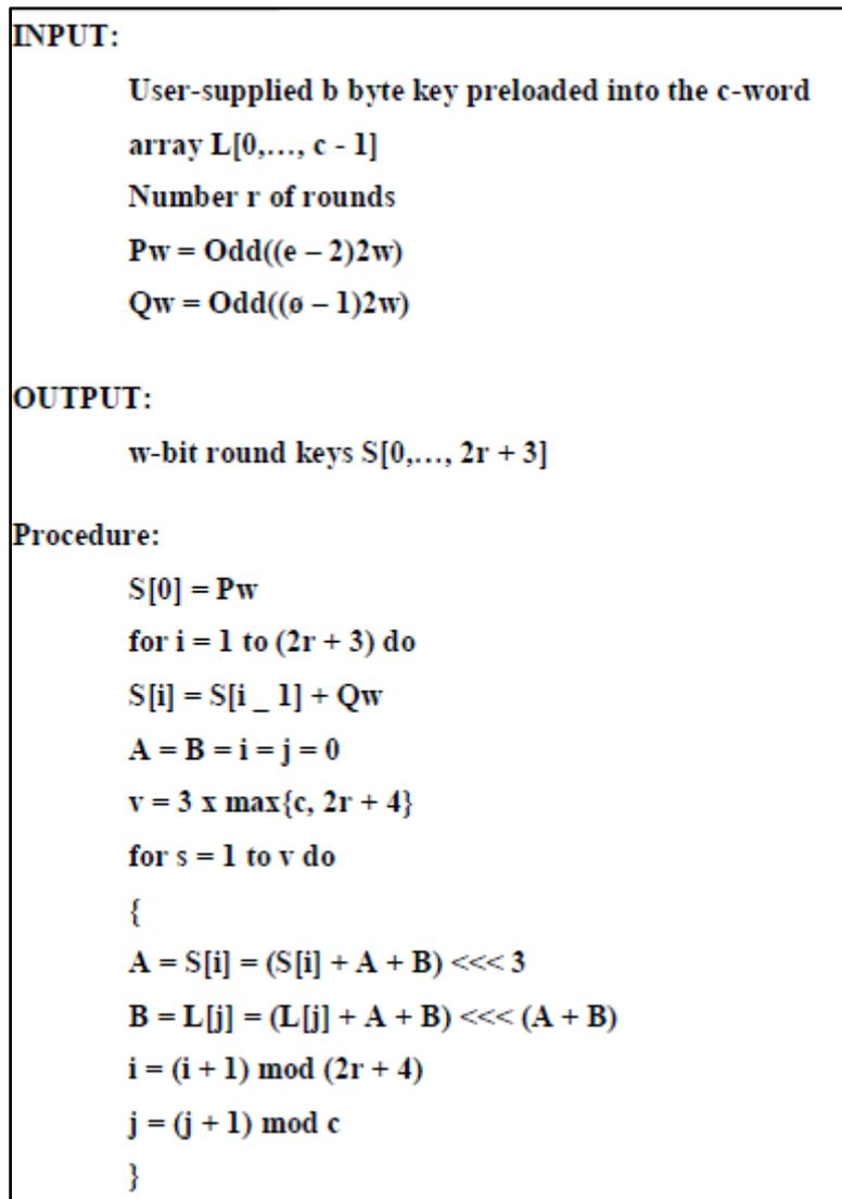
Figure3: key expansion algorithm of RC6 which is used in the proposed system
