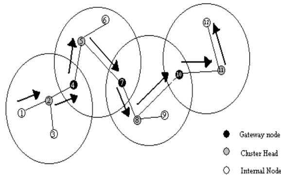
**Figure 4** Example of CGSR routing from node 1 to node 12
