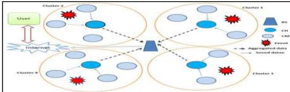
Fig. (2): Cluster-based Methodology in WSNs
