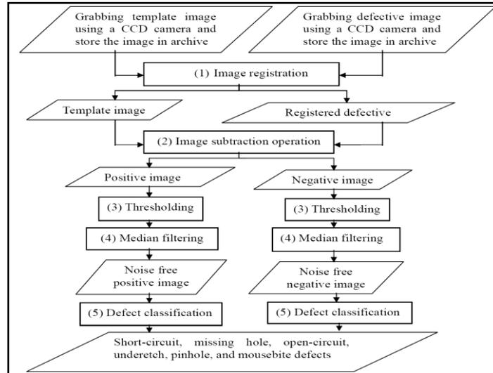
Figure 2. PCB defect detection flow chart
