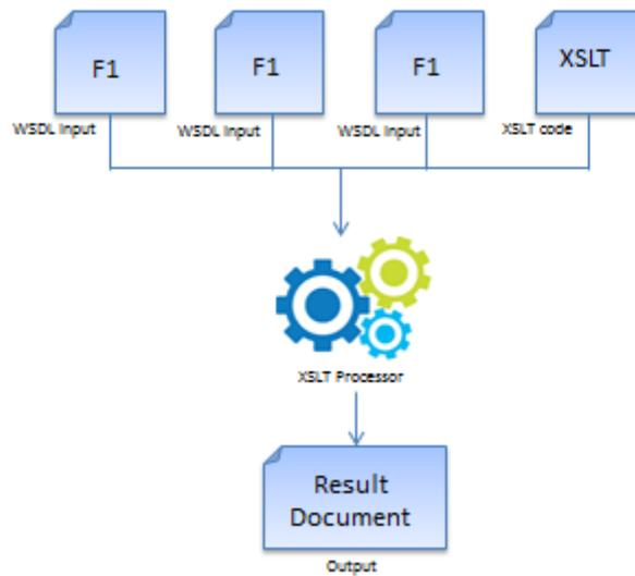
**Figure 2:** Operation of the XSLT Processor
