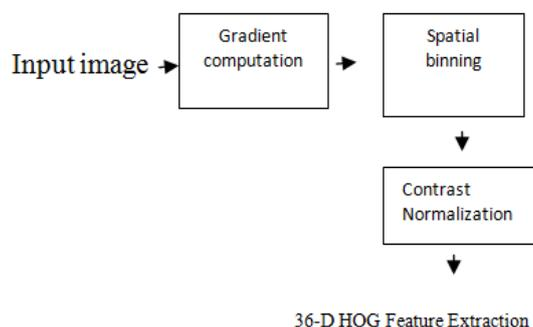
**Figure 2:** Block Diagram for extracting HOG from an input image
