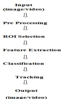
Figure 1: Flow diagram of major modules in vision based pedestrian detection system
