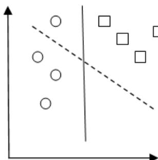
**Figure 3:** Hard-margin (solid line) and soft margin (dotted line) SVM Classifier
