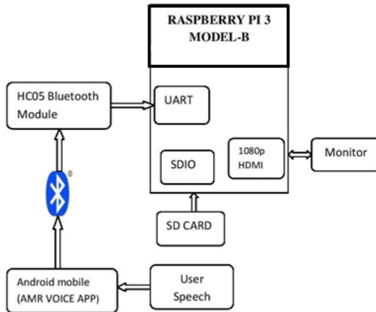
Figure 1: Block Diagram
